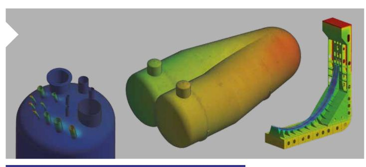
Direct coupled thermal structural analysis of cargo tanks and hull structure
