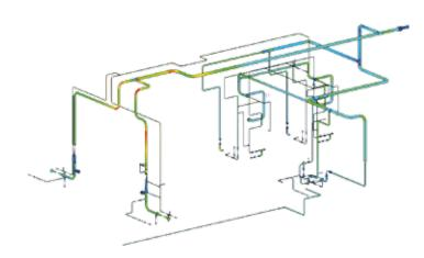
Pipe stress analysis of a LNG system
