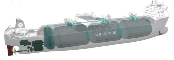
LEG carrier ECOSTAR 36k – triple-fuel, the world's first ethane driven LEG-Carrier, ready for LNG Our scope: Integration of fuel gas system and fuel gas tanks (tank foundation strength and temperature calculation, P&I diagram, 3D coordination, isometrics, pipe stress analysis)
