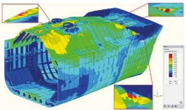
Detailed FE models for strength check of fore- and aftship transitions
