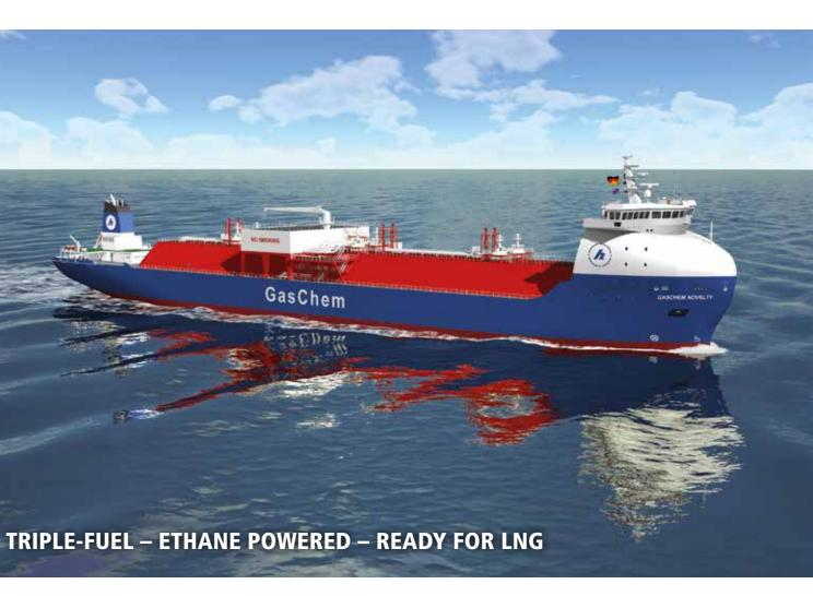
consumption. ECOSTAR 36K will be able to operate on HFO, MGO and, as a world novelty, on ethane. The fuel gas system is prepared for LNG and, if necessary, the ship can run on LNG as well. The vessel's autonomous gas fuel tanks are laid out for ethane and LNG and enable an operating range of about 10,000 nautical miles.
