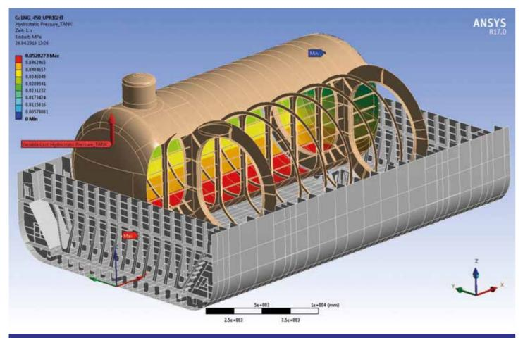
Interaction simulation of cargo tank and hull structure considering fix and sliding support and thermal contraction
