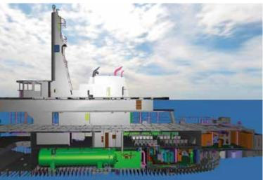
3D coordination model side view showing the fuel gas tank and
