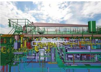
3D coordination model of ECOSTAR 36k, side view to compressor shelter
