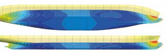
CFD results at design draught & speed. HB Hunte has developed in a constant cooperation with HSVA highly optimized gas tanker hull lines.
