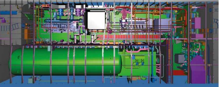
3D coordination model top view showing the fuel gas tank and fuel gas system
